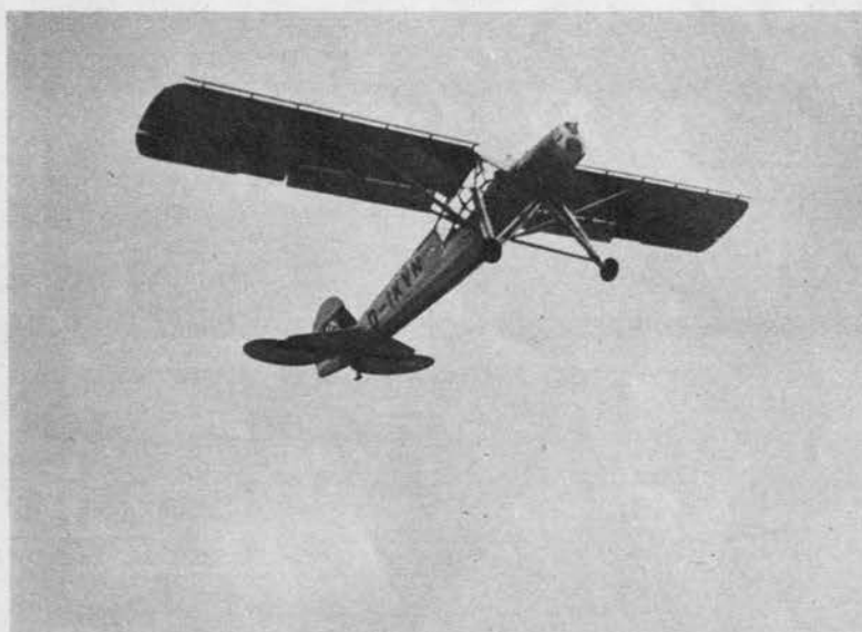
Squarish wingtips , long pointed nose and unique tailplane help distinguish Fieseler Storch from our observation craft. Rommel is said to have used a Storch with ambulance plane markings for flights in Lybia.
